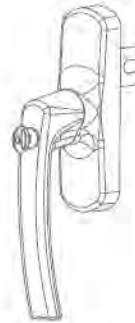
Anahtarlı eksenel kol Key locatable window handle
