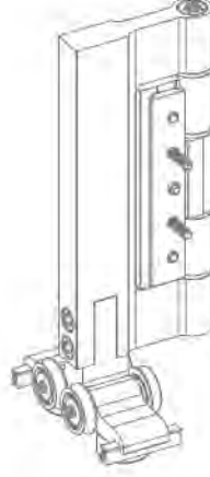
Çift Kanat Alt Rulman Double sash lower roller
