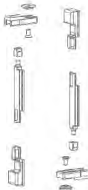
Kademeli teleskopik makas Stepped telescopic arm W55.743
